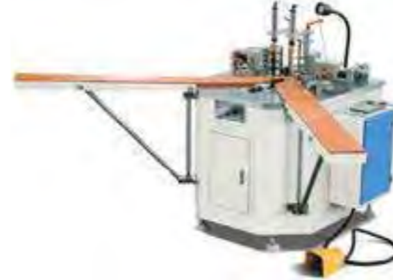
Single Head Corner Crimping Machine
