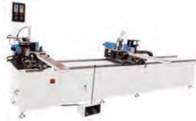
Double Head Corner Crimping Machine
